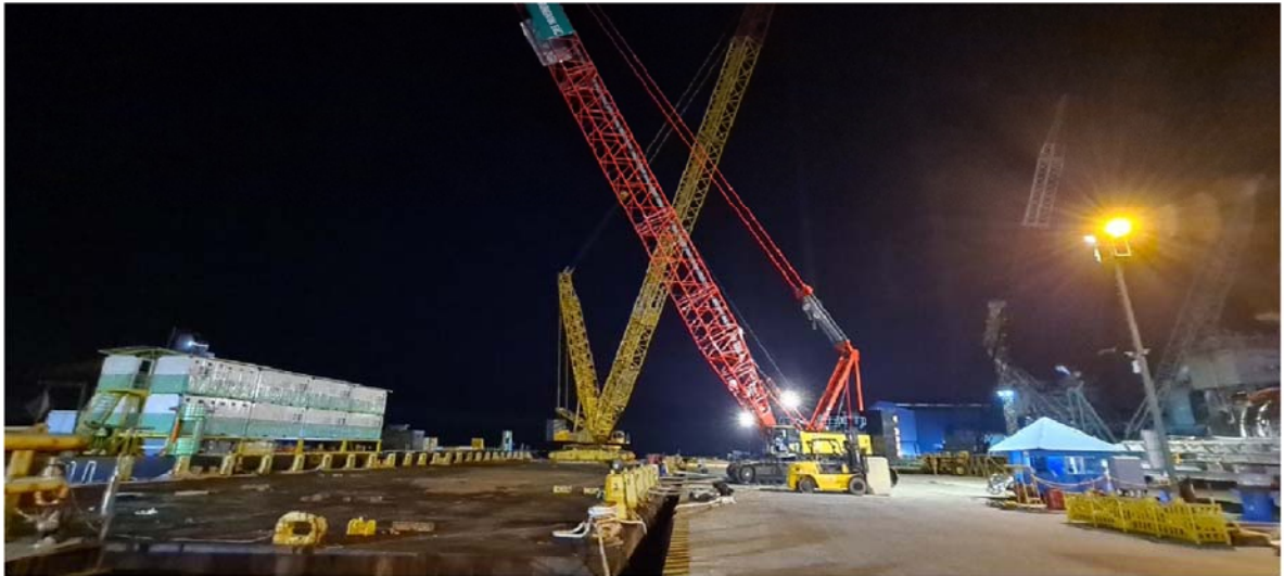
Roll-on Crawler crane to on barge
